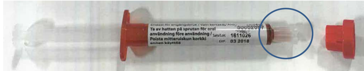
Figure 2. Upon removing the red cap, the translucent tip-cap remains on the syringe (abnormal removal reported) for illustrative purposes, not UK pack
